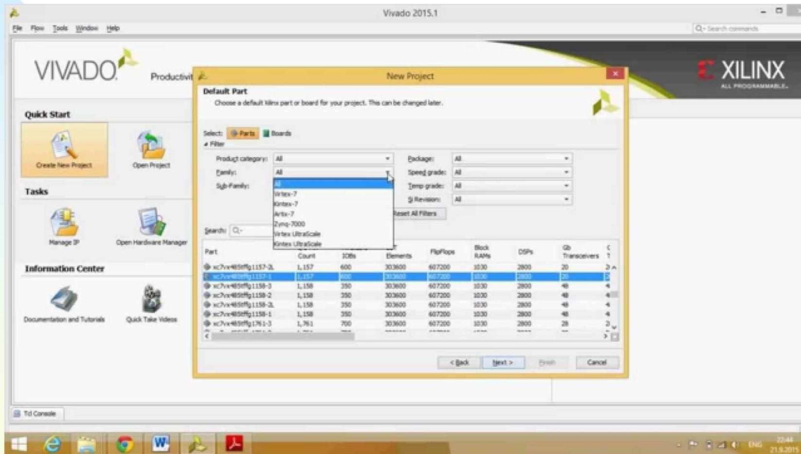
Define HDL project, target device, source files (if desired)
