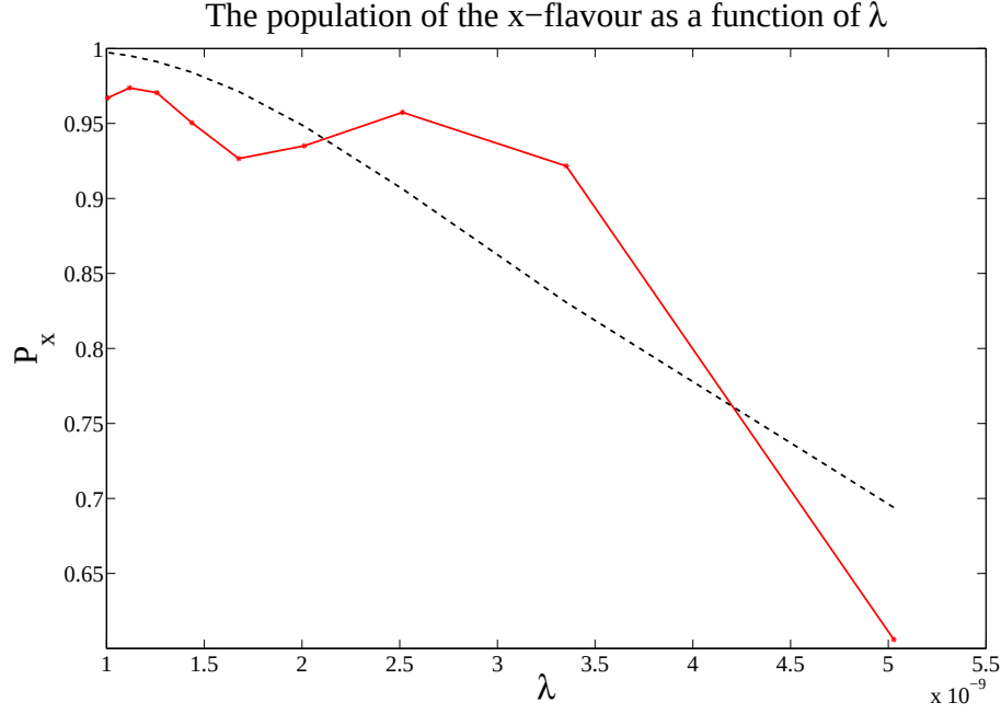
Figure 10: The figure depict how the population transition depends on \lambda (as define earlier). The red curve is the calculated points for the transition process with different \lambda 's. The black doted line is the fitting made from the Landau-Zener models prediction Eq.(113) with the adiabaticity parameter \Lambda as a fitting parameter. Note how for larger \lambda the process is less adiabatic and thus how fewer particles change from the starting state to the end state. Additionally, note how the fitting fails to capture the entire nature of the population transition processes. The figure is for the population difference p_x - p_y but as previously stated most of the particles should be in p_x therefore making p_y \approx 0 and the notation on the y-axis valid.
