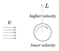
causes fluid velocity on one side to be higher than the other side. Then the force direction can be inferred from the application of Bernoulli's principle, or from the curvatures of streamlines on both sides of the cylinder.
