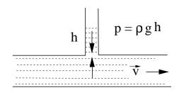
the pressure measured in a direction transverse to the flow (e.g., through the rise of liquid in a side tube) is the static pressure.
