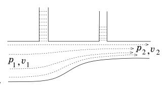
liquid in narrow side-tubes inserted at points 1 and 2) one can get information about the change in fluid velocity.
