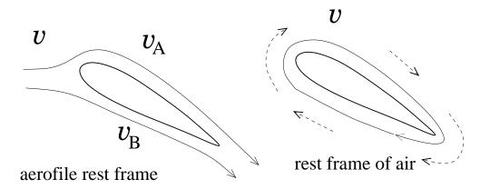
particles on the two streamlines, the velocity vectors give rise to a **circulation** around the aerofile in the clockwise direction <sup>3</sup>. Mathematically, the circulation is quantified by
