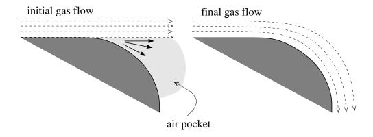
Instances of the Coanda effect are water falling on a vertically held curved surface or the bending down the air flow along the upper surface of an airfoil.
