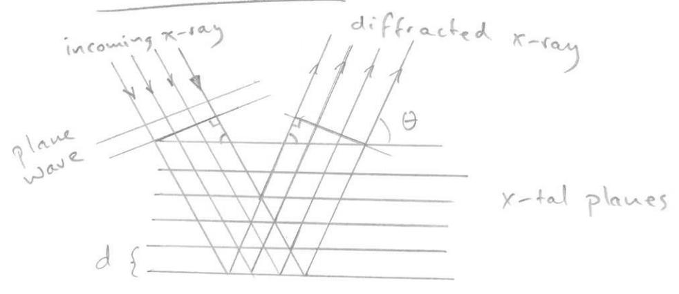
Diffraction  $\Leftrightarrow$  constructive interference
