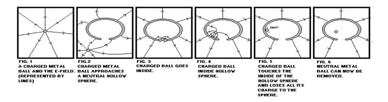
FIGURE 1. The charged metal bead is surrounded with an electric field. Don't be misled by the sparse "field lines," this field actually fills space completely and is not divided into widely separated lines. I drew the lines merely to show the intensity and direction of the field. Note that electric fields are measured in terms of volts per meter, so in a certain sense, an electric field is MADE of electric potential. We could say that an electric field IS VOLTAGE.
